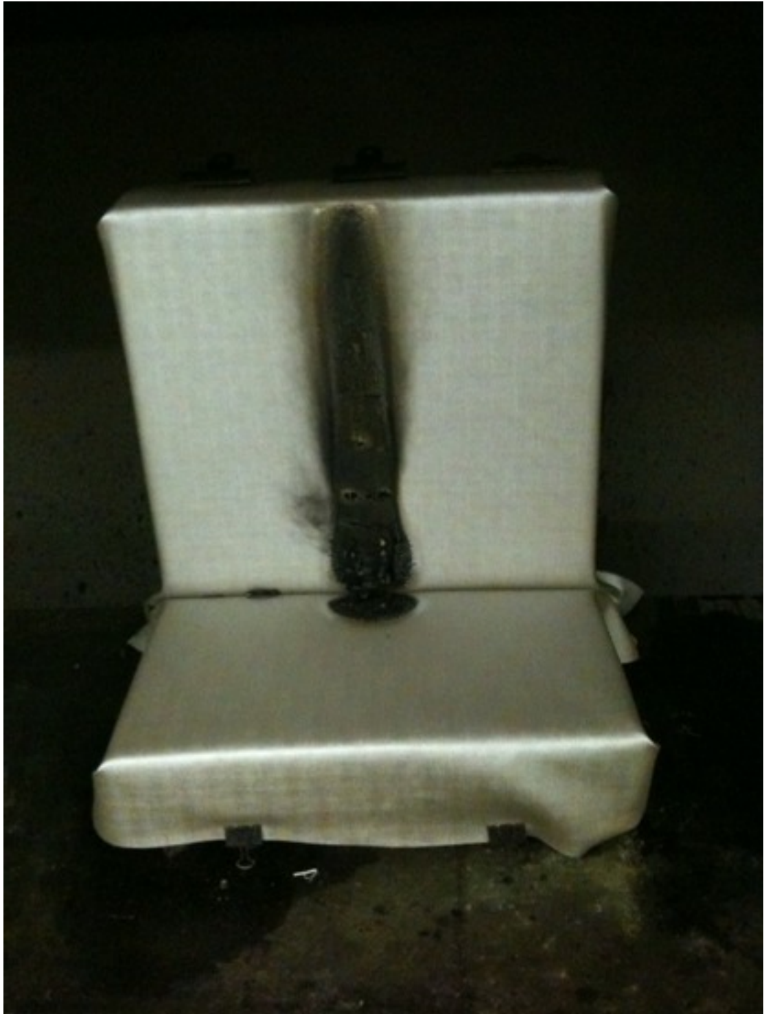
BS5852 Crib 5 Test – PASS
